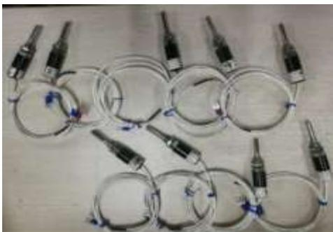
Fig 2: Pt100 temperature sensor
