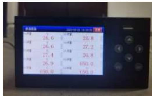
Fig 3: Multi-channel paperless recorder
